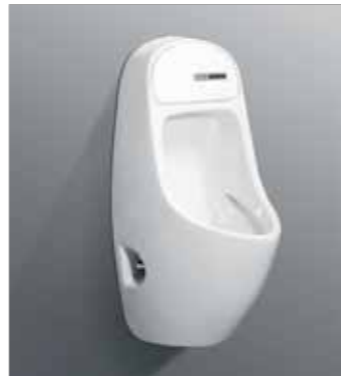
ø4010.0* Tamaro-S60B, siphonic urinal, with rear water inlet, with infrared proximity electronics, battery operated
